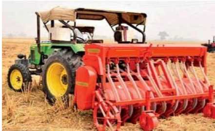
In-situ Paddy Straw Management using Happy Seeder – Wheat Seeding in standing paddy stubbles
