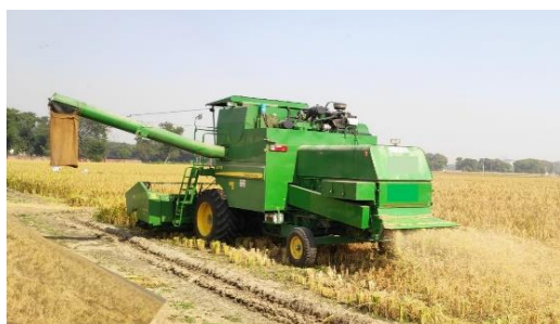
Combine harvester with Super Straw Management System (SMS)
