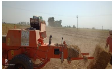
In-situ Paddy Straw Management using Happy Seeder – Wheat Seeding in standing paddy stubbles
