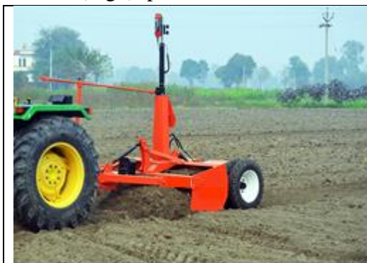
Fig 4: Laser leveler in operation
