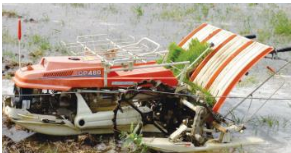
Fig 3. Walking type Mechanical rice transplanter (Source: Kumar et al., 2012)
