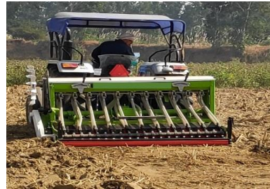
In-situ Paddy straw management using Super / Turbo Seeder – Incorporation of Straw into the soil
